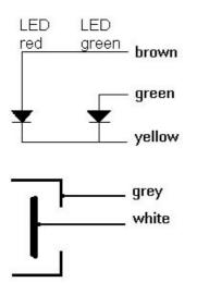
**Important**: Providing power source value higher than maximum value of  $V_F$  voltage (2,5 V for  $I_F$  = 20 mA) specified for LED is <u>not</u> recommended. If required – use the appropriate resistors for each type of LED.
